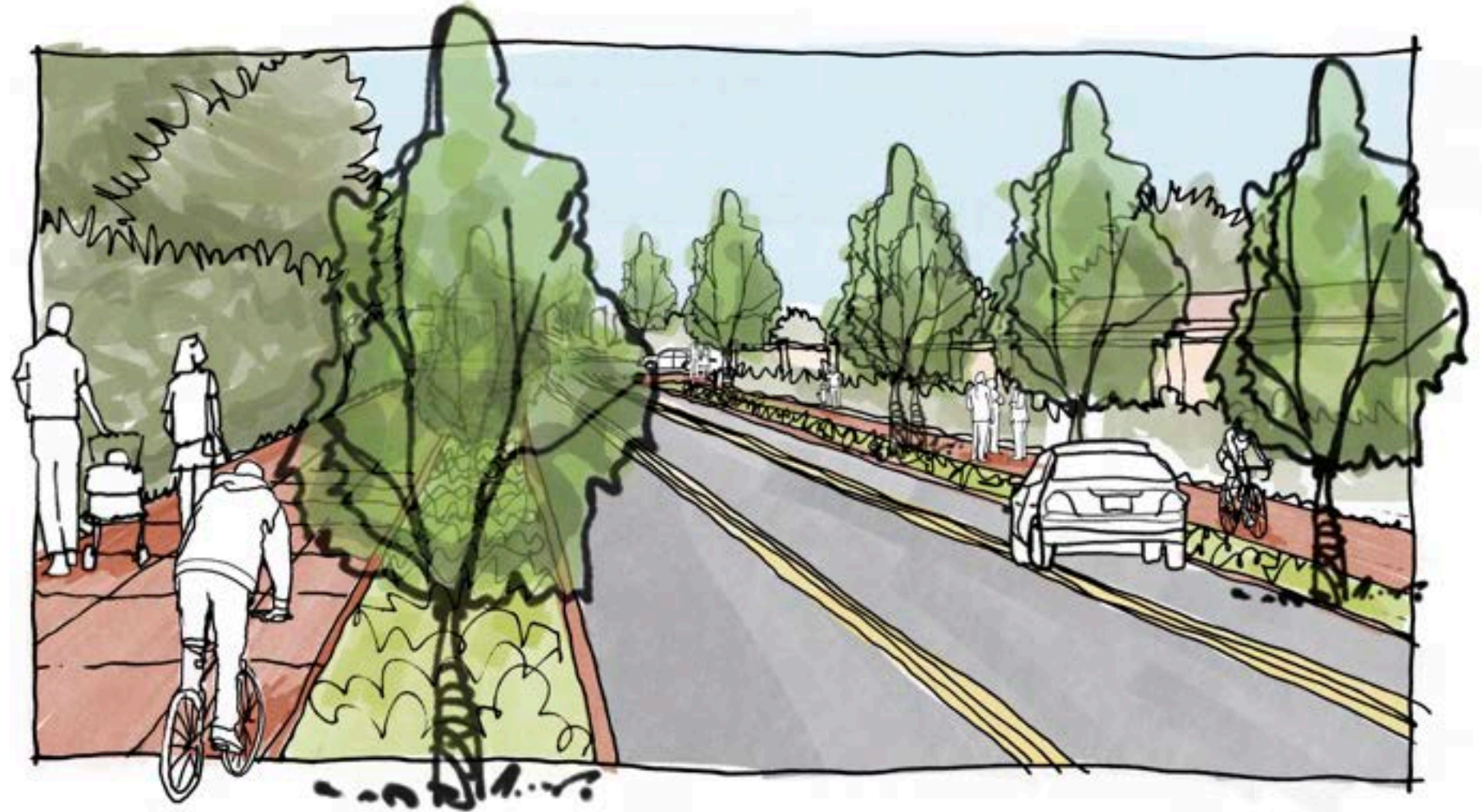
Conceptual rendering of an improved Washington Street, featuring a tree-lined, bike-and-pedestrian friendly narrowed roadway.
